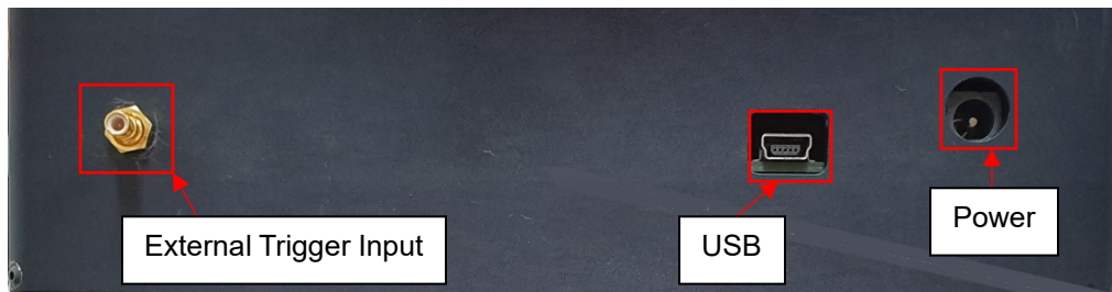
Figure 1. SM301-EX Backside Panel
